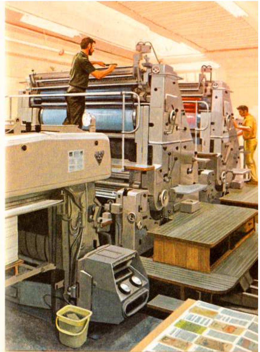
The four-colour offset litho machine that printed this book. Sheets making two complete Ladybird books are printed in a double journey through the machine, four colours in quick succession on each side of the sheet.
