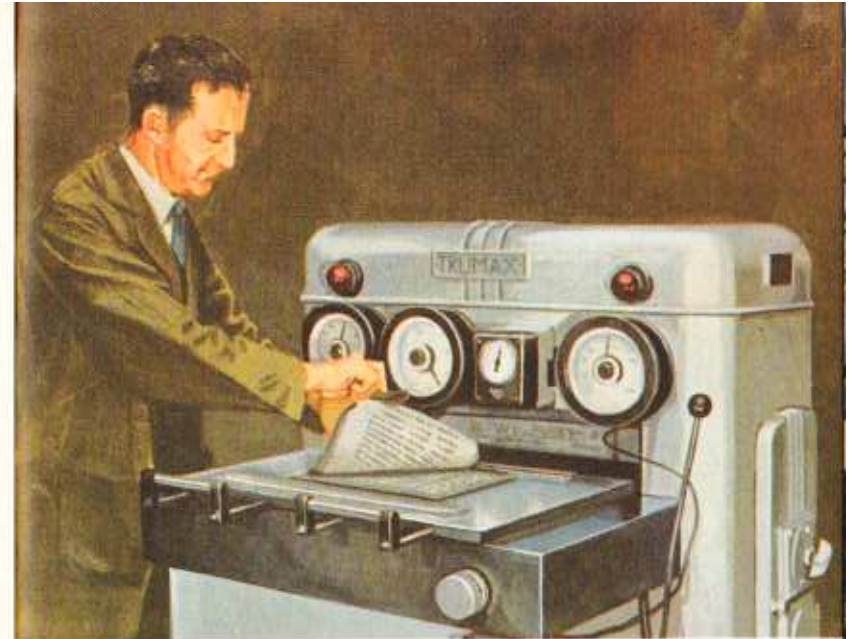
Pulling a moulded stereo off the matrix. This machine is used for producing matrices for stereos and electros and for moulding rubber or plastic stereos.
